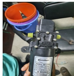
Figure 5. Water flow pump
